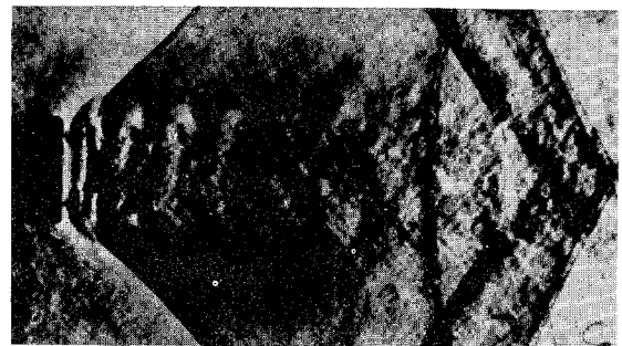
a) Toroidal vortex shedding, H_j/H_\infty = 1.10
