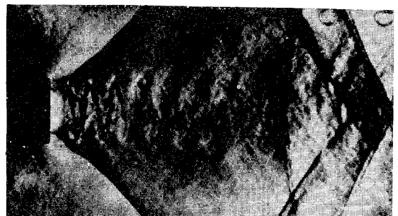
b) Helical vortex shedding, H_j/H_\infty = 1.31
